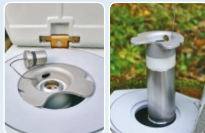
By using HT well caps and intermediate rings, the Datalogger is unable falling down in the borehole
