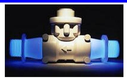
This multi-range radial flow turbine meter uses a low inertia turbine supported on robust sapphire bearings in a chemically resistant housing. Ten flow ranges (0.01 to 160 litres per minute), a choice of "plug in" fittings and individual traceable calibration make this meter one of the most flexible available. For OEM applications the fittings can be tailored to suit the installation and speed production. Custom leads or connectors are also available for quantity orders.
